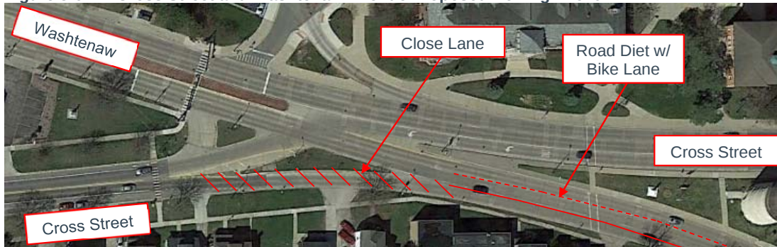
Figure 5-6 Cross Street and Washtenaw Avenue Proposed Re-Alignment
