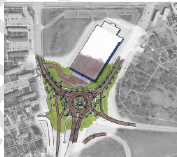
Figure 14: Roundabout for Two-Way Conversion
