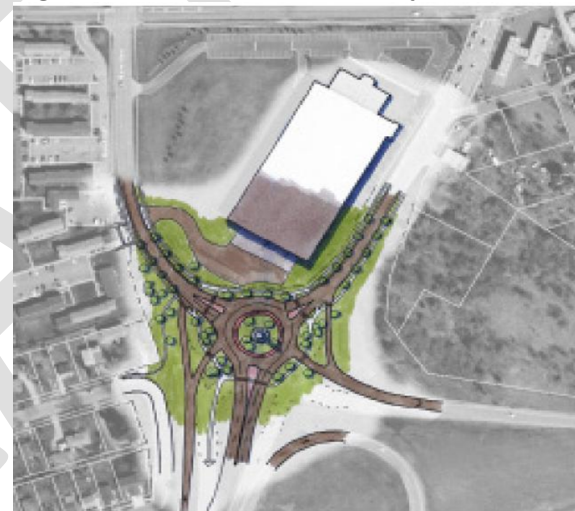
Figure 14: Roundabout for Two-Way Conversion
