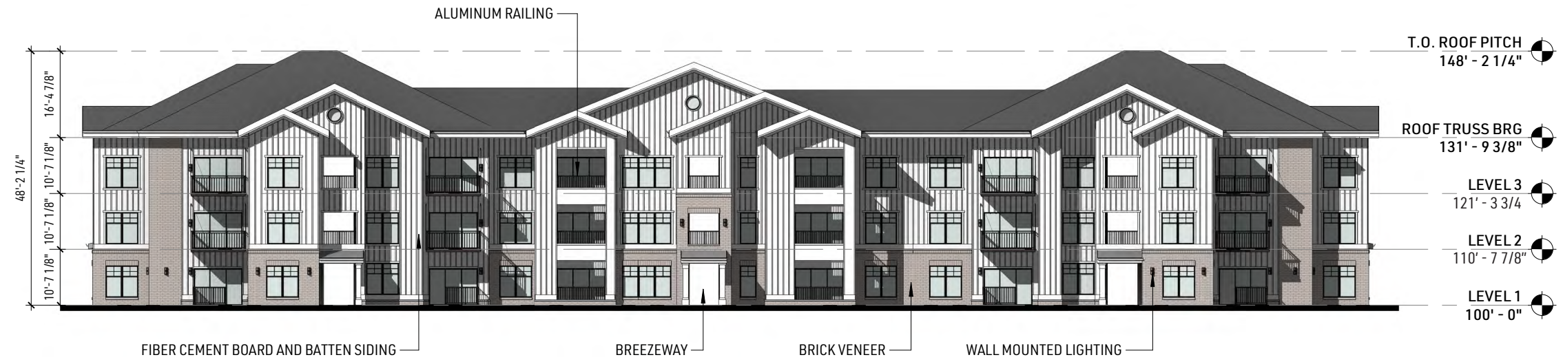
NORTH & SOUTH ELEVATION 3/64" = 1'-0"
