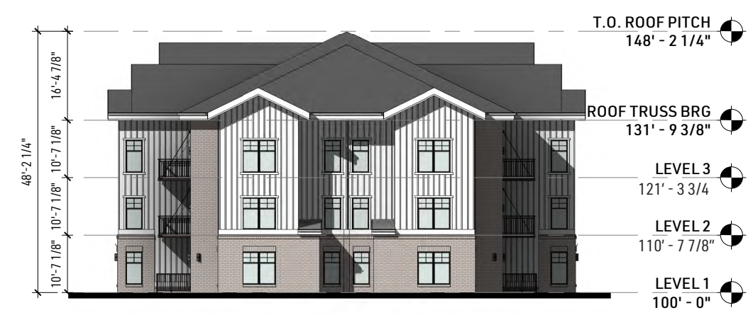
EAST & WEST ELEVATION 3/64" = 1'-0"
