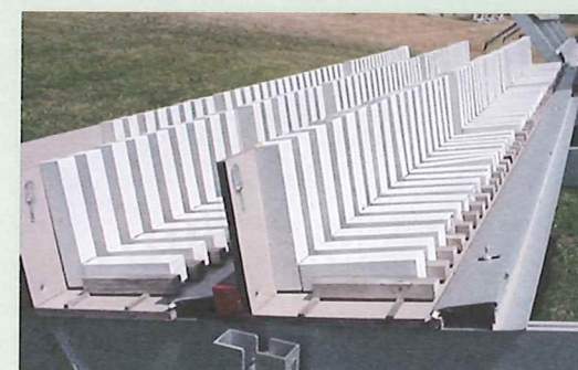
"L-Joint" visual appearance environmental test
