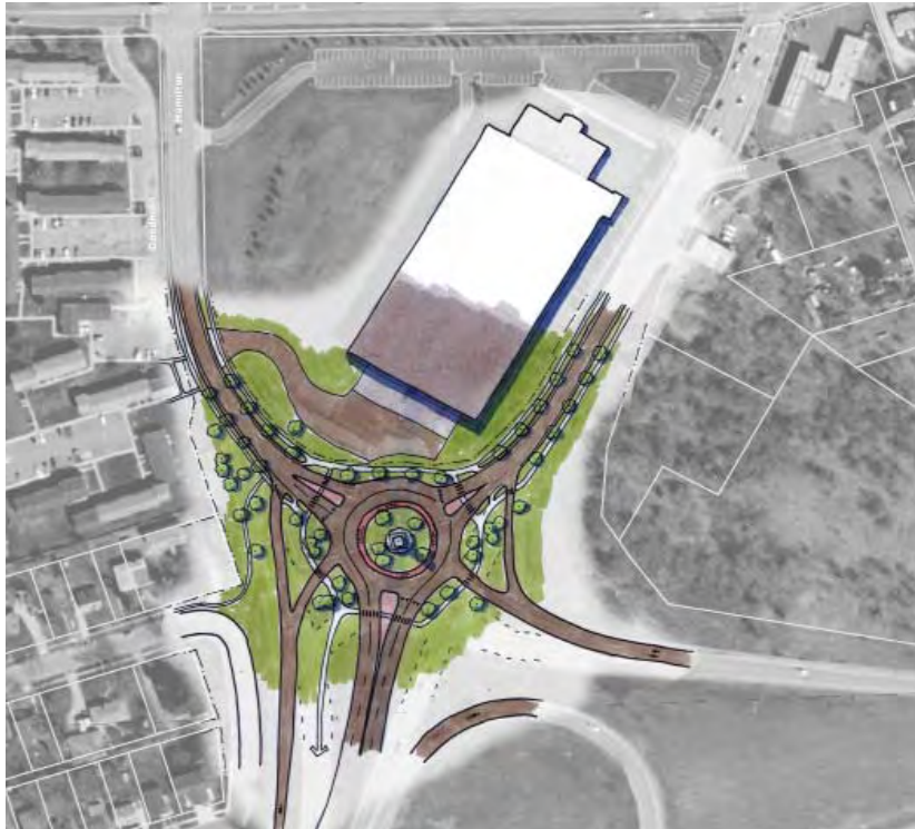
Figure 15: Roundabout for 2-Way Conversion
