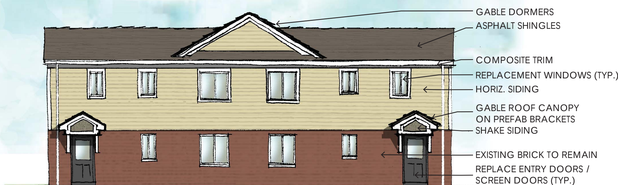
REAR ELEVATION - BUILDING 'D' 1/8" = 1'-0"
