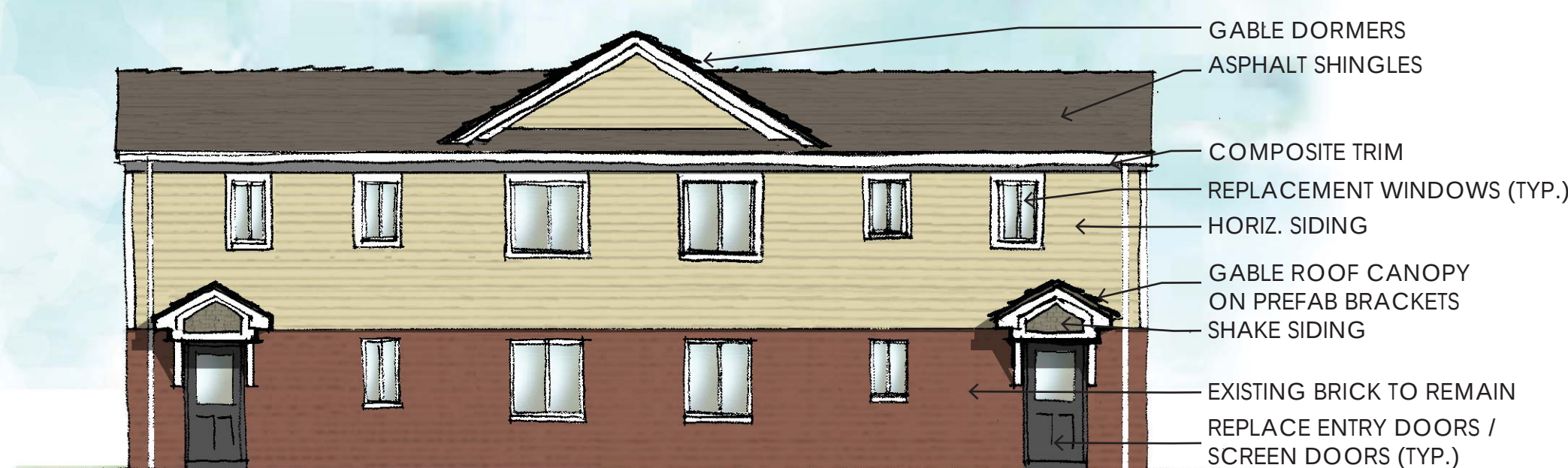
REAR ELEVATION - BUILDING 'D' 1/8" = 1'-0"
