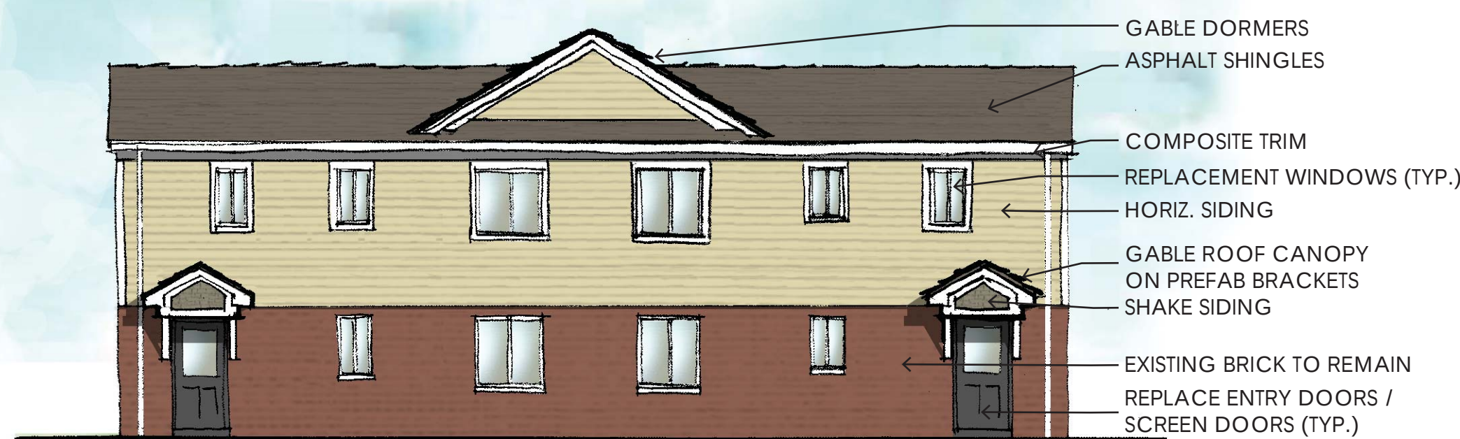
REAR ELEVATION - BUILDING 'D' 1/8" = 1'-0"
