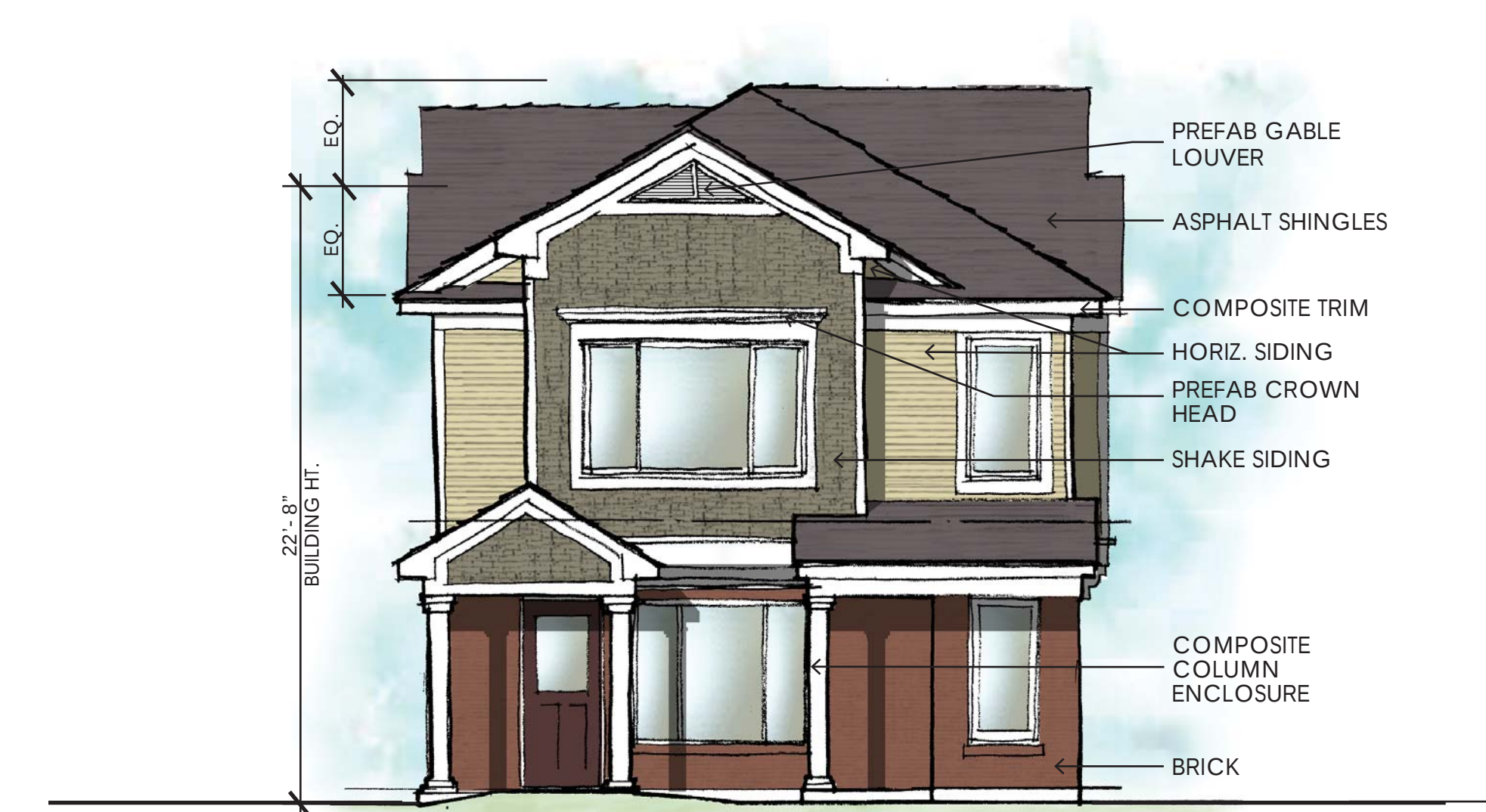
FRONT ELEVATION (BLDGS 723,729) 3/16" = 1'-0" 2 BEDROOM UNITS - STACKED
