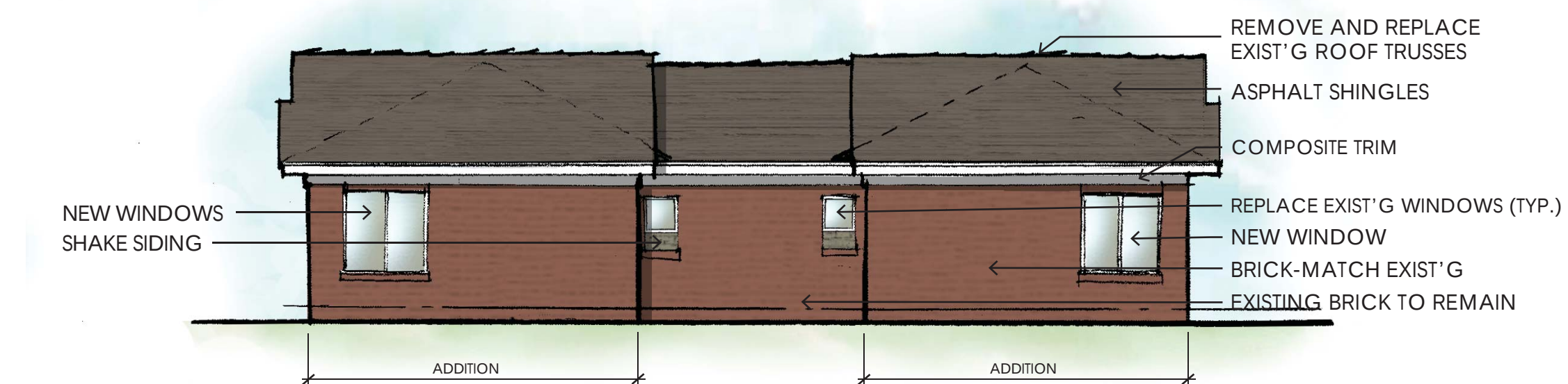
REAR ELEVATION - BUILDING 'C'
