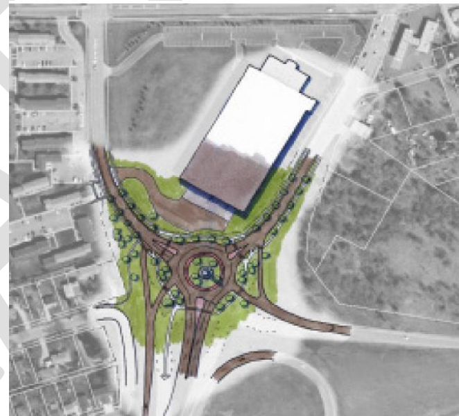
Figure 14: Roundabout for Two-Way Conversion
