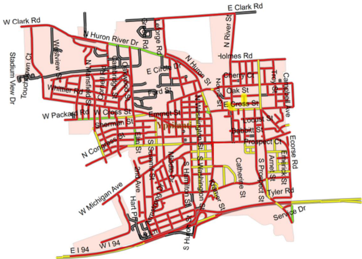
Figure 1: Map showing location of Ypsilanti's paved roads (i.e., those managed by Ypsilanti) and their current condition for paved roads with green for good (i.e., PASER 10, 9, 8), yellow for fair (i.e., PASER 7, 6, 5), and red for poor (i.e., PASER 4, 3, 2, 1), as well as the location of Ypsilanti's unrated roads in grey
